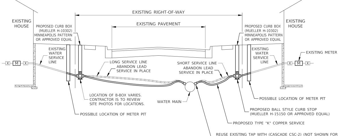
REUSE EXISTING TAP WITH (CASCADE CSC-2) (NOT SHOWN FOR CLARITY) 1BALL STYLE CORP STOP (MUELLER H15000 OR APPROVED EQUAL)
