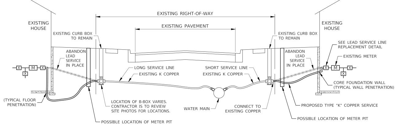
NOTE: ① ONLY CURB BOXES THAT ARE NOT FUNCTIONING ARE TO BE REPLACED PER THE SPECIAL PROVISIONS. ANY CURB BOXES THAT ARE BURIED SHALL BE ADJUSTED PER THE SPECIAL PROVISIONS.
